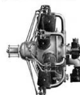
Outside and cutaway views of the Marchetti 8-cylinder, 135 h.p. radial type construction airplane engine.
